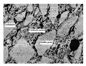
Fig. 1. Micrograph of cordierite mullite refractory.
