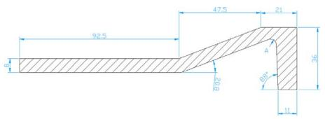
Fig. 2. Geometry of the refractory models.
