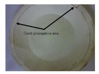
**Fig. 3.** Typical cracking scheme in refractories.
