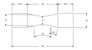
Fig. 1. Shape and dimension of mechanical testing specimens
