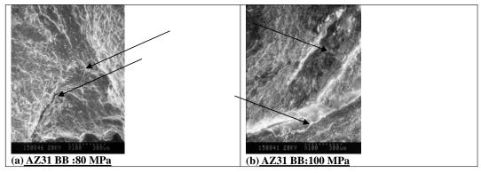
Fig. 5. SEM micrographs showing cracked surfaces at difference stress for BB at (a) 80MPa; (b) 100 MPa
