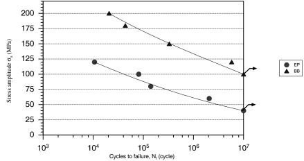
Fig.2. S-N curve for rolled AZ31 at EP,BB conditions, rotating beam, R=-1, 50Hz.
