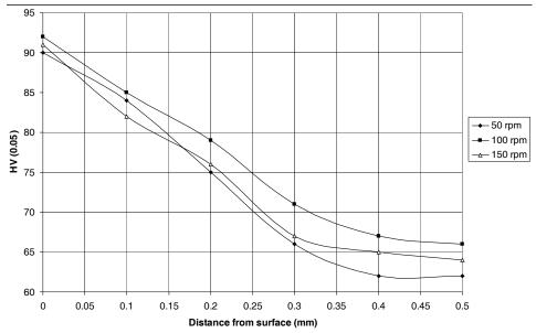
Fig. 3. Microhardness profile oif AZ31 after BB at 200 bars, 0.17 mm/min at different BB rotation speed.
