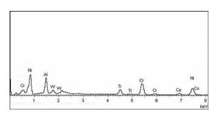
**Fig. 8.** EDS analysis of the outer coating layer in L-1050 sample: (a) zone I, (b) zone II, indicate that zone I is rich in Al while zone II is rich in Ni.
