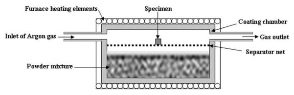
Fig.1. Schematic showing the coating equipment used for the gas phase aluminizing process
