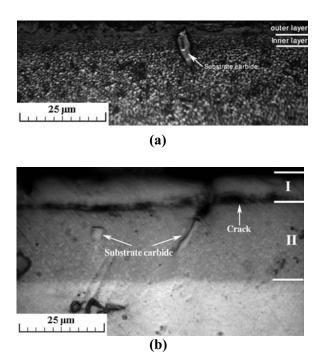
Fig. 5. Optical image of the coating formed by (a) pack L, (b) pack H, at 850°C, showing the substrate carbides within the outer coating layers
