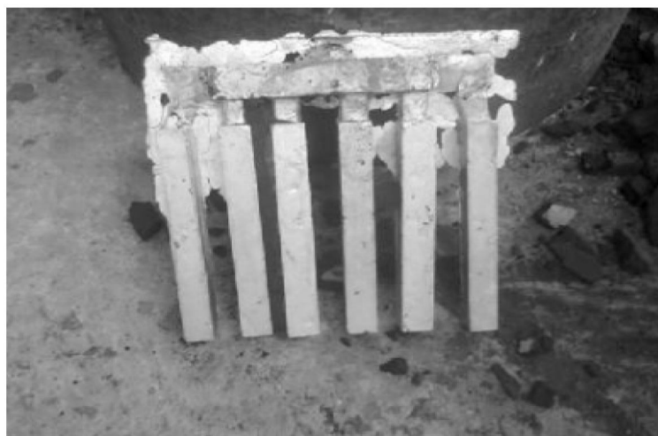
Fig.1. Green/ Dry Sand Casted samples (size of cast 1x1x8 in)
