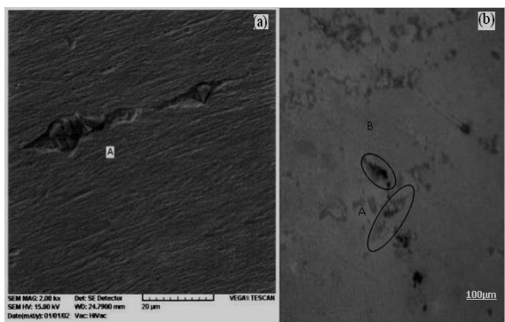
Fig. 14. Formation of inter-metallic compounds in microstructure of matrix phase for spring steel 1.4568 after heat treatment (at 480°C , 80 min and cooling in air, then heating in oil bath 230°C for 60 min and cooling in cold water) and respectively (a) Scanning Electron Microscopy (SEM) (b) optical microscopy.
