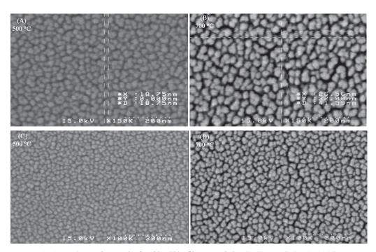
Fig. 3. FE-SEM micrograph of a  $TiO_2$ – $SiO_2$  films annealed at (A,C) 500 °C, (B,D) 700 °C.
