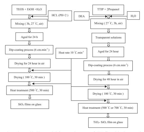
**Fig. 1.** Experimental procedure used in this research (left: preparation process of SiO2 films, right: the preparation process of TiO<sub>2</sub>-SiO<sub>2</sub> films).
