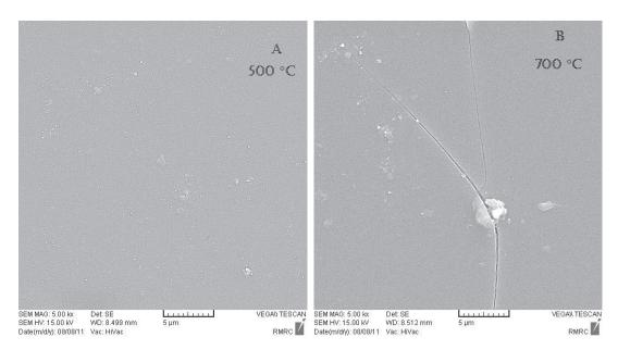
Fig. 2. SEM micrographs of  $TiO_2 - SiO_2$  films prepared in annealing temperature (A) 500 °C (B) 700 °C
