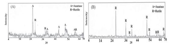
Fig. 4. XRD patterns of TiO<sub>2</sub>-SiO<sub>2</sub> films produced on glass Substrates annealed at (A) 500 °C and (B) 700°C for 30 min in air.
