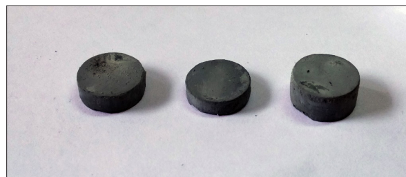
Fig.2. compacted pure silicon after pressing
